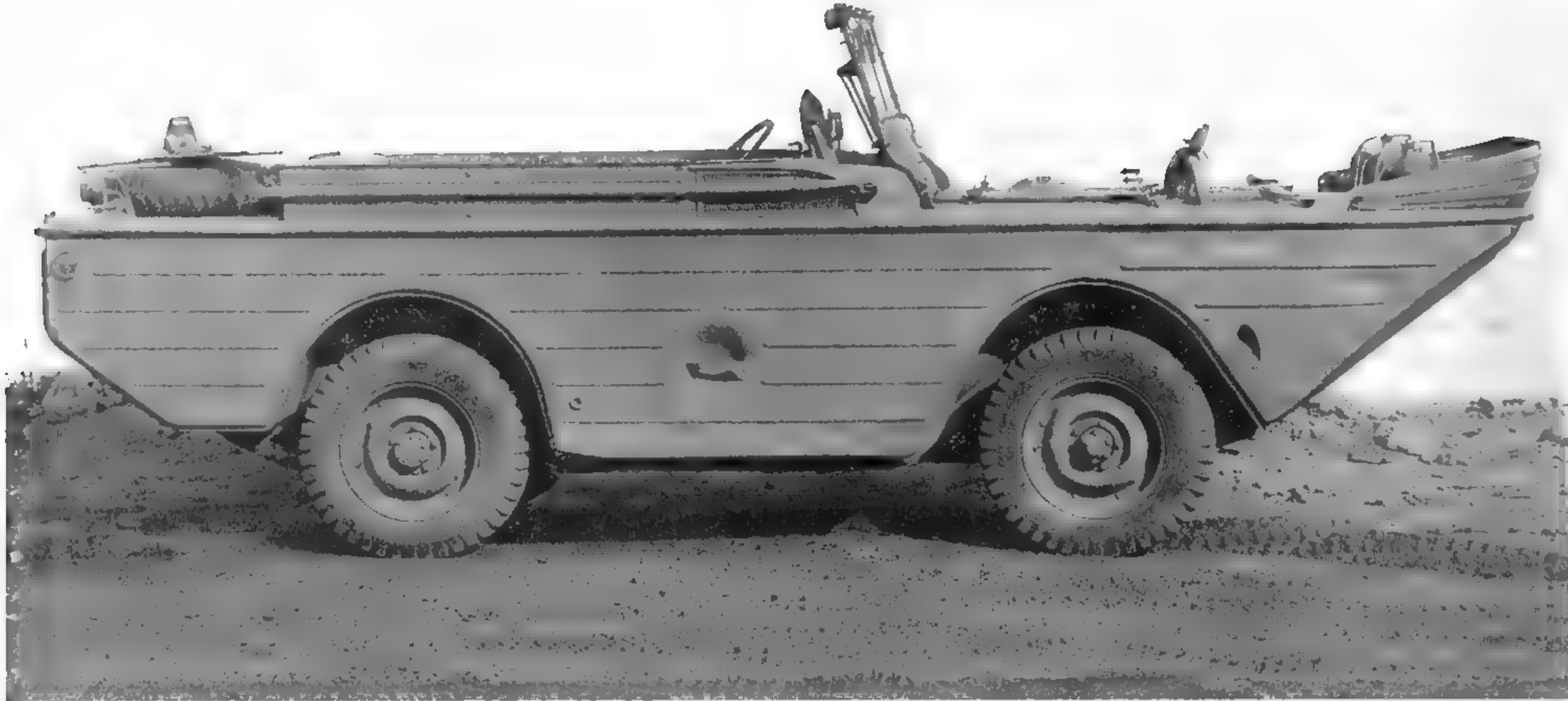
The engine-cooling door has been closed in this photo, but the hood itself can just be made out ahead of the windshield. Alongside the passenger compartment is the boat hook (pike pole) that was released as standard equipment for the GPA vehicles on Dec. 27, 1942. (U.S. Army photo)
